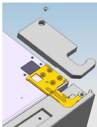
b. Use a tool to remove the 4 screws off the upper hinge cover and then remove the latter.
