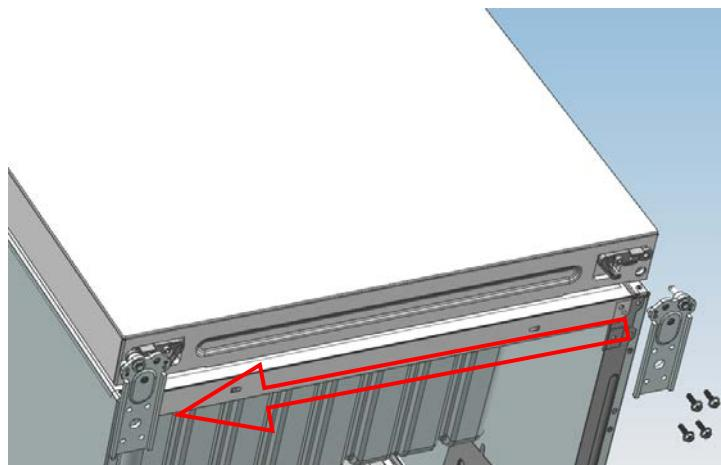
b. Assemble the shorter adjustable front foot to the lower hinge side and adjust the height of the foot to make the refrigerator stay in level.
