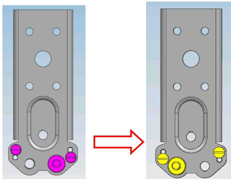
三： Assemble the refrigerator door and freezer door to the opposite side.
