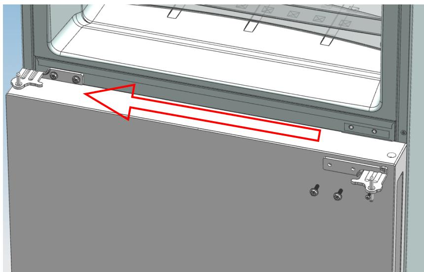
3. Put on the refrigerator door and assemble the left upper hinge to the other side of the cabinet; use a tool to screw up the 4 screws to fix the upper hinge.
